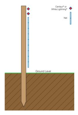
When installing wire above stock netting we would recommend using one or two strands of Centaur® or White Lightning®.
