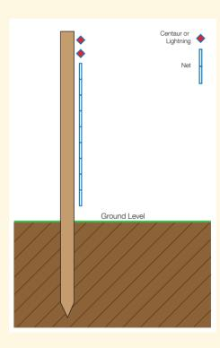
When installing wire above stock netting we would recommend using one or two strands of Centaur or Lightning.
